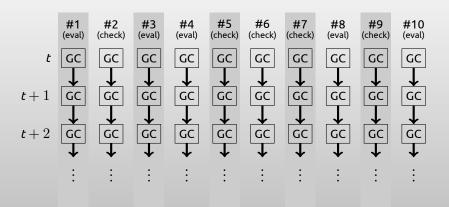
sender generates garbled circuits, reusing wire labels within each thread
