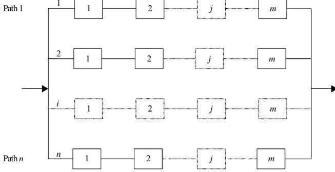
Figure 2. Conceptual Network of Parallel-Series System
